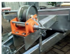
Fig. Option: Winch + cable + brace
